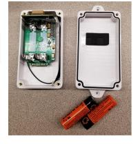
4. Replace the batteries ensuring that they are placed properly-match the + and -
